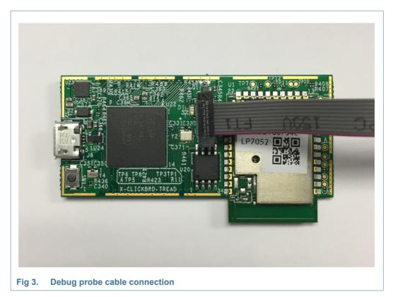
Power the module by connecting to it to a power supply or PC via J8. Note that when the 802.11 module is transmitting, the current drawn may be several hundred milliamperes. So, a power supply capable of delivering more than 500 mA is recommended.
