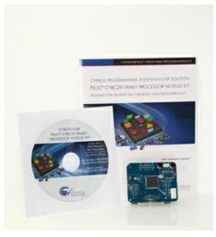
This processor module can be used in conjunction with the PSoC Development Kit (CY8CKIT-001) to create designs utilizing on-board DVK resources or compatible expansion boards. This kit provides you with an additional processor module to use with different projects.
