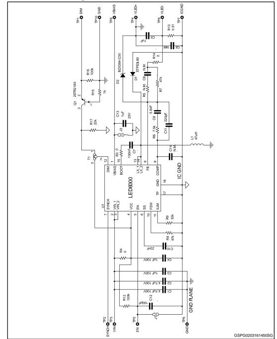
Figure 1: STEVAL-ILL079V1 circuit schematic
