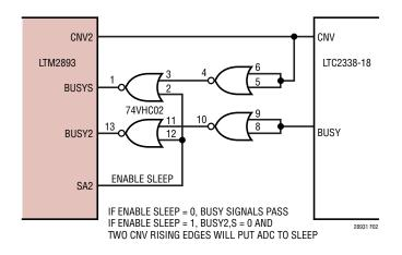
Figure 2. ADC Keep-Alive and Sleep Enable
