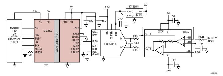
Figure 14. Isolated 1Msps LTC2378-18 Single-Ended OV to 5V Input (BUSYS = GND2)
