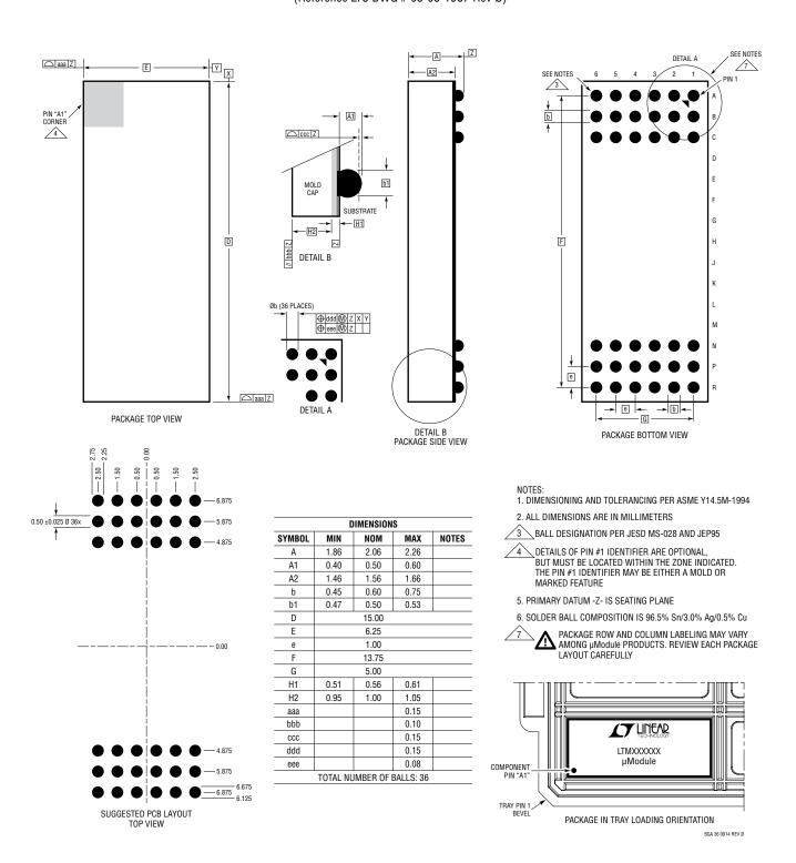
**BGA Package 36-Lead (15mm × 6.25mm × 2.06mm)** (Reference LTC DWG # 05-08-1987 Rev Ø)
