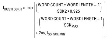
where  $t_{BUSYFSCKR}$  is the time between the falling edge of BUSY and the 1st rising edge of SCK, SCK2 is the nominal configured frequency in Hz and SCK\_MAX is the maximum frequency in Hz.
