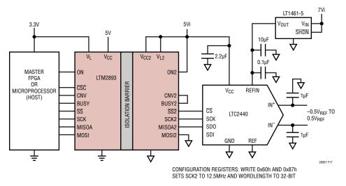
Figure 17. LTM2893 with LTC2440 Delta Sigma ADC
