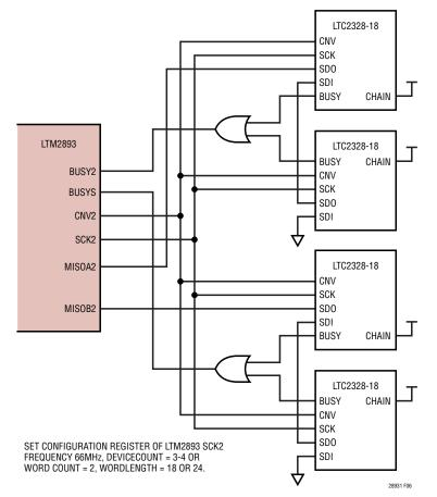
Figure 6. Connecting Four ADCs, One Chain Into MISOA2 and One Chain Into MISOB2
