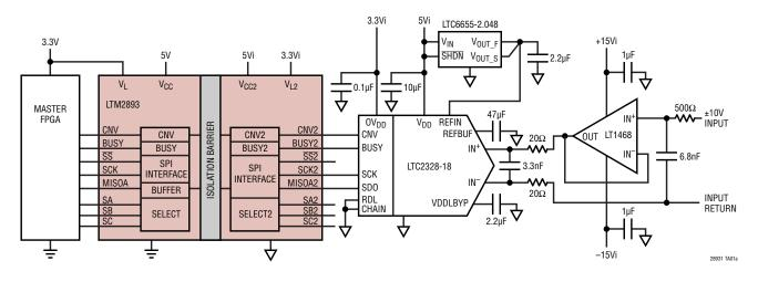
LTC2328-18 ADC Isolation  $A_{IN} = \pm 10.24V$ , SNR = 95dB
