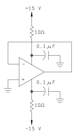
FIGURE 2. Radiation exposure circuit.
