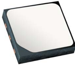
Figure 7. Si7022 with Factory-Installed Protective Cover
