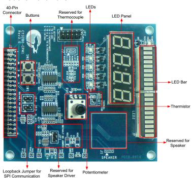
The module board consists of an LED panel, a potentiometer, an LED bar, six LEDs, a thermistor, and two buttons. These are interfaced to the CapSense Controller board via a 40-pin receptacle connector (J2). The board also consists of two loop-back connection jumpers (JP3 and JP4) to demonstrate the variable length SPI master-slave communication.
