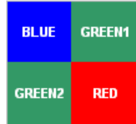
Figure 6. Color Filter Arrangement on the Pixels
