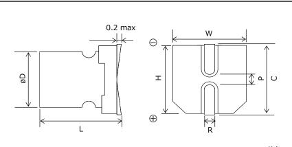
Unit : mm Size L +0.1 -0.4 øD±0.5 W±0.2 H±0.2 C±0.2 R P±0.2 code C6 6.3 5.9 6.6 6.6 7.3 0.6 to 0.8 2.1 E7 8.0 6.9 8.3 8.3 9.0 0.6 to 0.8 3.2 7.9 F8 10.0 10.3 10.3 11.0 0.6 to 0.8 4.6 E12 8.0 11.9 8.3 8.3 9.0 0.8 to 1.1 3.2 F12 10.0 12.6 10.3 10.3 11.0 0.8 to 1.1 4.6
