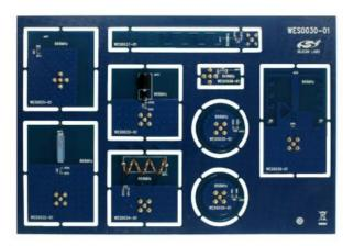
individually as well. The panel contains a mix of PCB, chip and wire antenna options for a specific frequency band.
