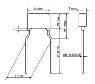
Coating extension does not exceed the end of the lead bend.
