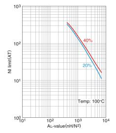
The 20% and 40% graph shows when a 20% and 40% drop from the initial AL-value has been made due to the DC superimposition.
