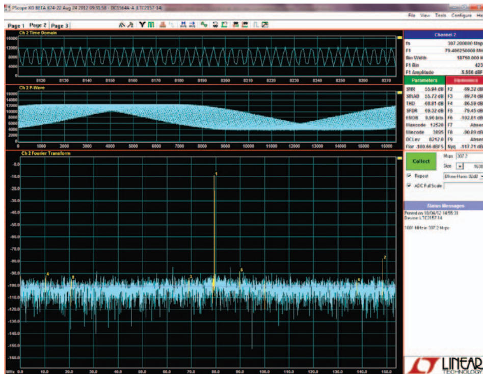
Figure 7. ADC Output: 1-Tone Test at 1000MHz with 307.2Mps Sampling Rate Undersampled in the Seventh Nyquist Zone
