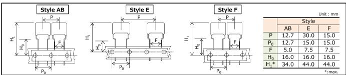
\*: H1 dimension is based on insertion machine "Panasert RH series" made by Panasonic. Consult with Panasonic technical staff when using other insertion machines.
