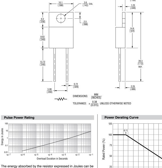
The energy absorbed by the resistor expressed in Joules can be calculated by multiplying the peak power of the pulse in watts times the length of the pulse in seconds.
