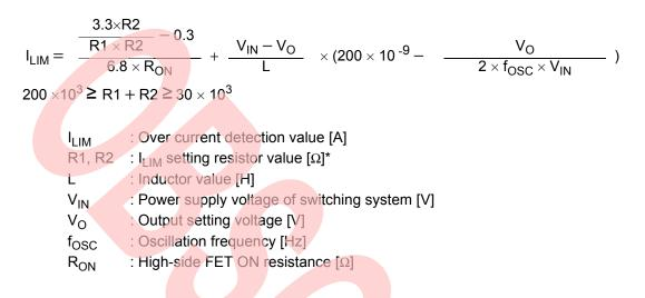
\* Since the over current detection value depends on the on-resistance of FET, the over current detection setting resistor value ratio should be adjusted in consideration of the temperature characteristics of the on-resistance. When the temperature at the FET joint part rises by + 100 °C, the on-resistance of FET increases to about 1.5 times.
