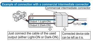
Note: Ensure to insulate the unused output wire.
