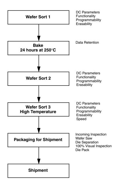
Figure 1. AMD KGD Product Test Flow
