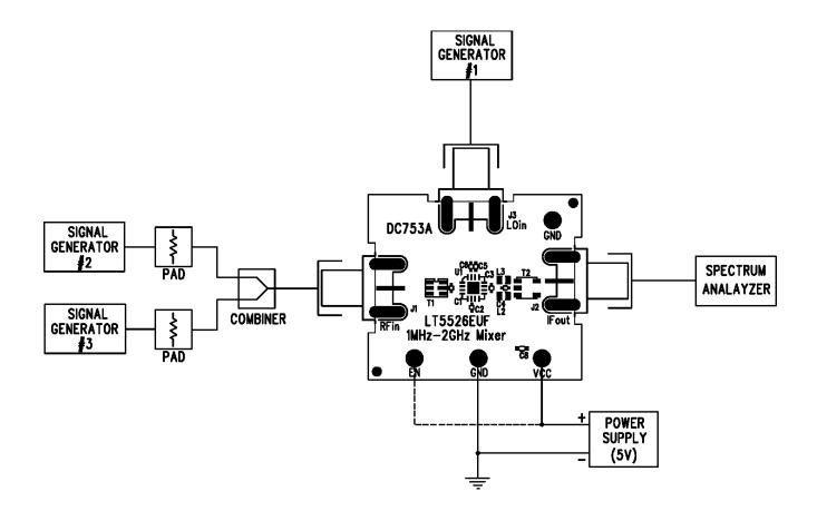
Figure 1. Proper Measurement Equipment Setup
