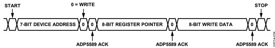
Figure 27. I 2 C Single-Byte Write Sequence
