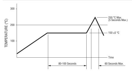
Processing Method: Reflow soldering with infrared heat or forced air convection (only once).
