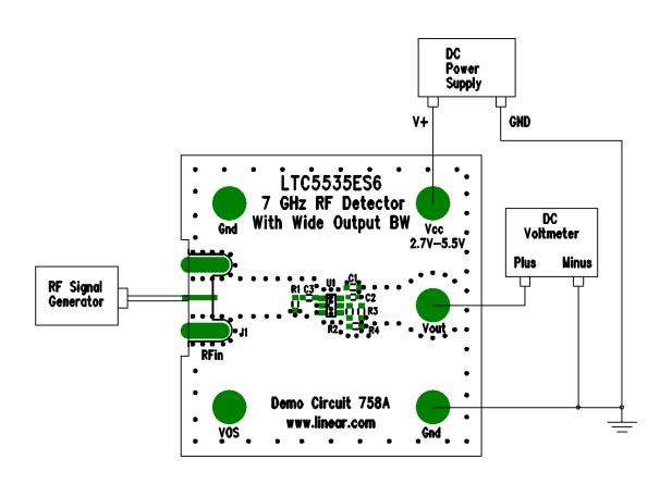
Figure 1. Proper Measurement Equipment Setup
