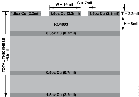
Figure 17. Evaluation Board (Cross Section View)
