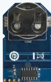
Si4010 EZRadio® KEY FOB TRANSMITTER
