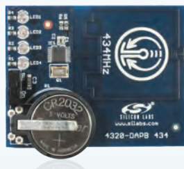
Si4320 WIRELESS REMOTE CONTROL DEMO BOARD
