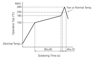
Reflow temperature may vary by location even in the same reflow condition. Please check the reflow temperature at terminals and at the top of a switch to make sure the both temperatures are within the specification. If even one of them is out of the specifications, please adjust.
