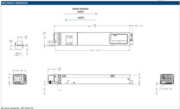
AC input connector: IEC 320-C14
