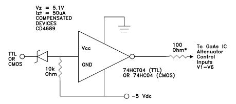
Simple driver using inexpensive standard logic ICs provides fast switching using minimum DC current.
