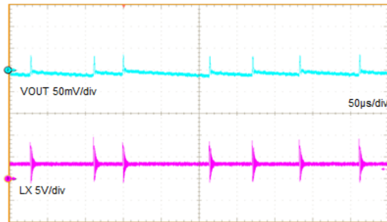
Figure 9-10 Switching waveform (VIN=7.4V, Iout=0.05A), LPM at SLP_N=L
