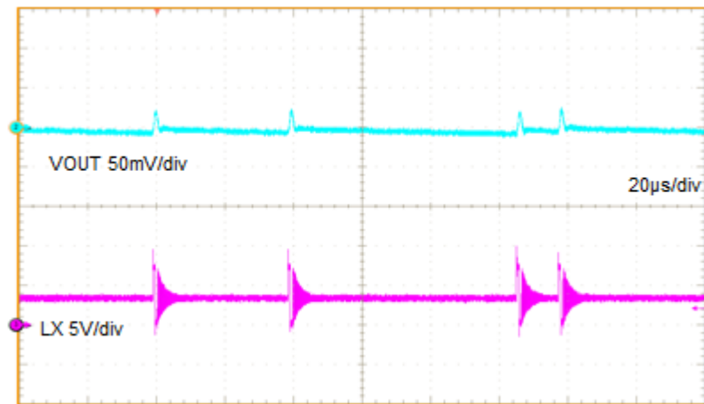
Figure 9-8 Switching waveform (VIN=7.4V,Iout=0.05A) , SLP_N=H
