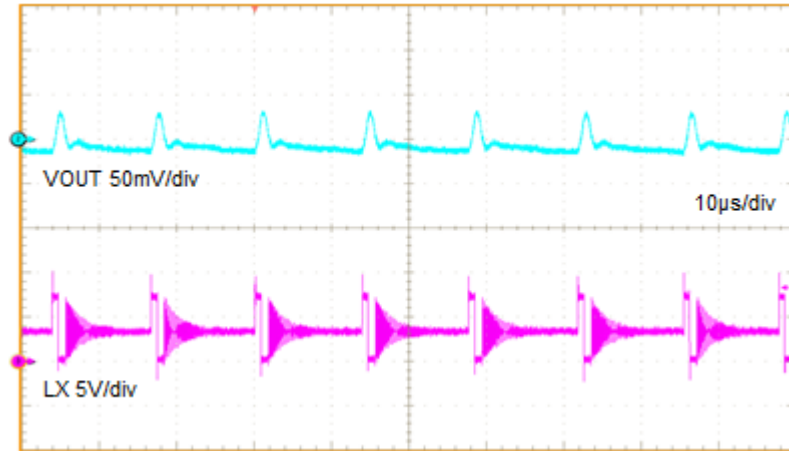
Figure 9-9 Switching waveform (VIN=7.4V, Iout=0.3A), LPM at SLP_N=L
