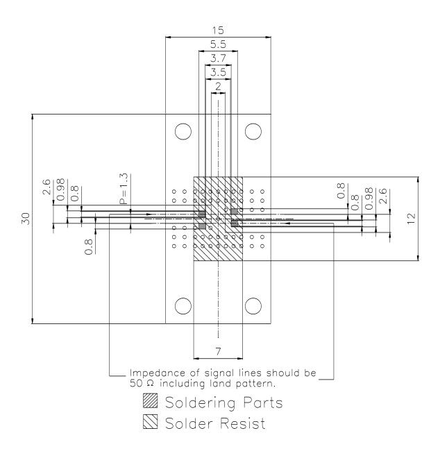
Note: Impedance of signal lines should be 50 ohms including land pattern. This standard condition is applying to the BT resin board (t = 0.4, dielectric constant = 3.6, copper plating on both surfaces).
