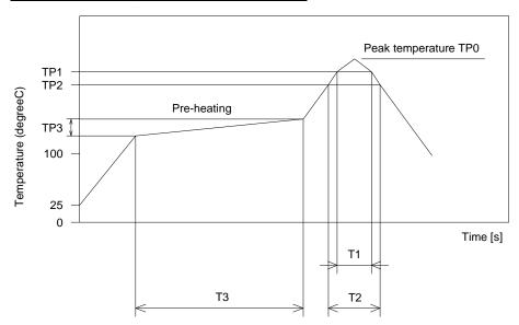
Measuring point of temperature: IN-OUT Terminals of The Device
