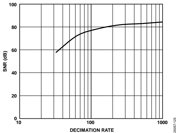
Figure 31. SNR vs. Decimation Rate of Sinc3 Filter Order
