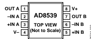
Figure 3. 8-Lead SOIC_N (R-8)
