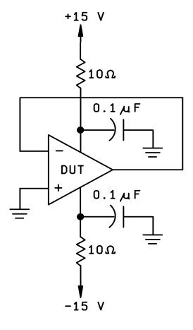
FIGURE 2. Radiation exposure circuit.
