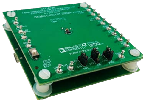
Figure 7. DC2662A mounted on top of DC2661A
