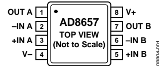
Figure 1. AD8657 Pin Configuration, 8-Lead MSOP
