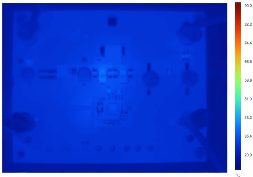
Figure 12. DC2814A-A Thermal Performance at 8V IN (Buck-Boost), 8V OUT , 3A Load Current
