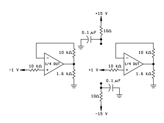
FIGURE 2. Radiation exposure circuit.
