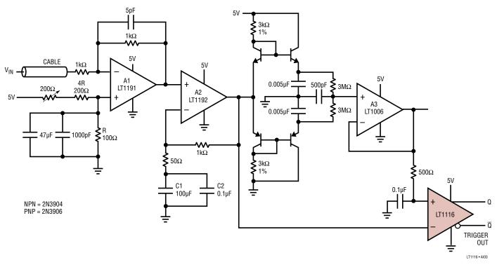
Figure 3. Fast Single Supply Adaptive Trigger
