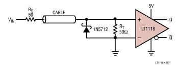
Figure 1. The Zero Crossing Detector Terminates the Transmission Line at Its  $50\Omega$  Characteristic Impedance. Negative Inputs Should Not Fall Below –2V to Keep the Signal Current Within the Clamp Diode's Maximum Forward Rating. Positive Inputs Should not Exceed the Device's Absolute Maximum Ratings nor the Power Rating on the Terminating Resistor
