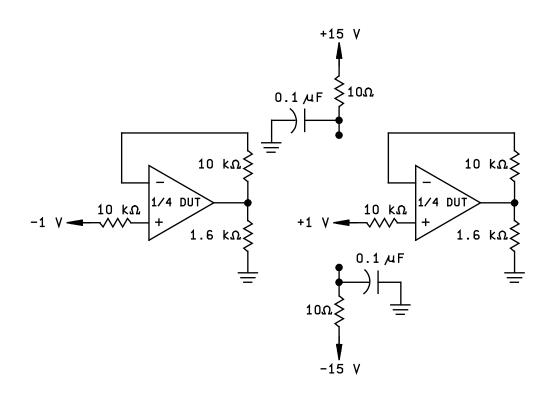
FIGURE 2. Radiation exposure circuit.
