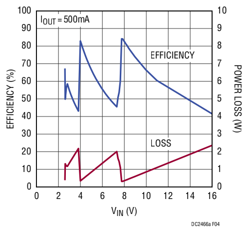
Figure 4. 3.3V Efficiency and Power Loss vs Input Voltage
