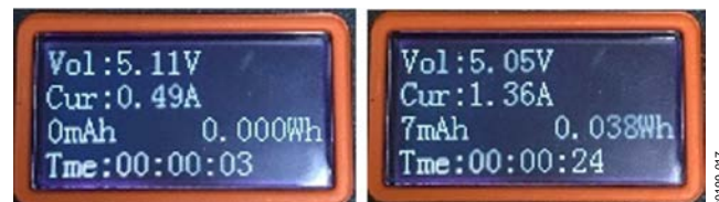
Figure 17. ET910 USB Multimeter Tester Screenshot of Phone A Charging from the Top USB Port (Left) vs. the Lower Port with the DCP Controller (Right)
