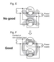
3) Terminal (2)-(6) (screw terminal (2)-(3)) should be connected as the start input. Connect terminals (2)-(7) (screw terminal (2)-(4)) for reset signal input. Connect terminals (2)-(5) (screw terminal (2)-(5)) for stop signal input. Be sure not to connect with other terminals and apply excessive voltage. The internal circuit will be damaged.
