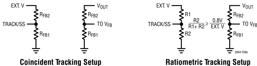
Figure 9(b): Setup for Ratiometric and Coincident Tracking
