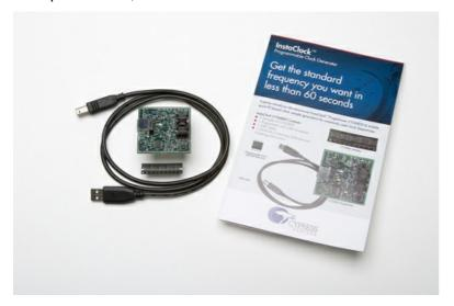
The CY36800 InstaClock Universal Programmable Clock Generator Programming Kit contains the programming board with a USB cable, and 3 samples each of the CY22800 and CY22801 devices. You can order more samples of either CY22800 or CY22801 Online. The latest programming software is available to download from www.cypress.com/instaclock.
