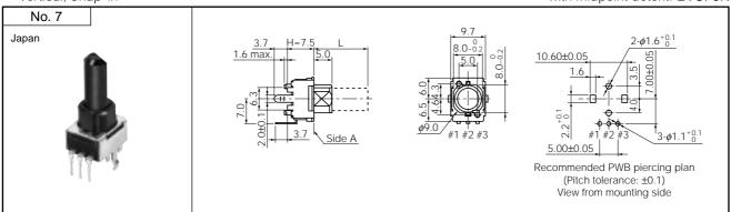
without midpoint detent: EVUF2L Vertical, Snap-in with midpoint detent: EVUF3L
