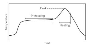
For soldering (Example: Sn/Pb)
