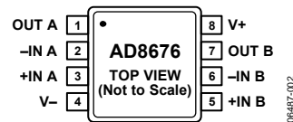
Figure 2. 8-Lead MSOP (RM-8)
