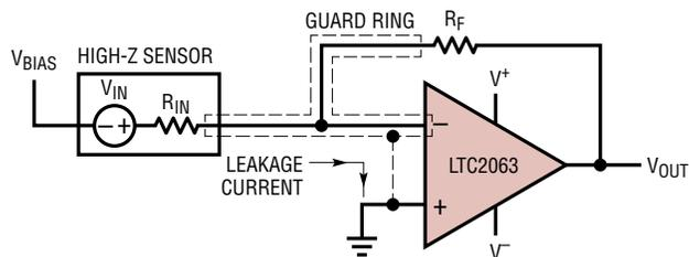
LEAKAGE CURRENT IS ABSORBED BY GROUND INSTEAD OF CAUSING A MEASUREMENT ERROR.
