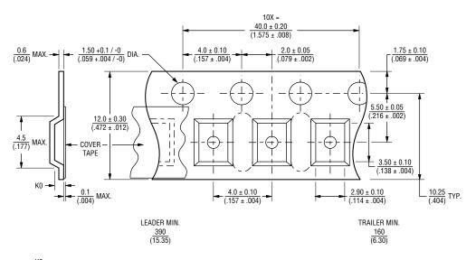
K0  $0.65 \pm 0.10$  MF-USML175/6 ~ MF-USML260/6, MF-USML175/12 ~ MF-USML260/12  $\frac{1.10 \pm 0.10}{0.023 \pm 0.004}$  MF-USML300/6 ~ MF-USML700/6, MF-USML300/12 ~ MF-USML550/12
