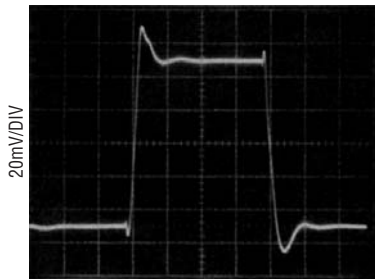
Small-Signal Transient Response V_S = \pm 2.5V
