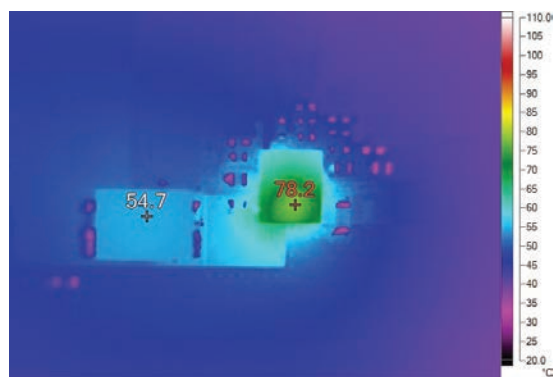
Figure 5. Thermal Picture ( V_{IN} = 12V , I_O = 20A . 21°C Ambient, No Forced Airflow)
